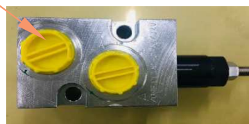
② Counter balance valve block
