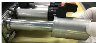
② Disassemble coil
